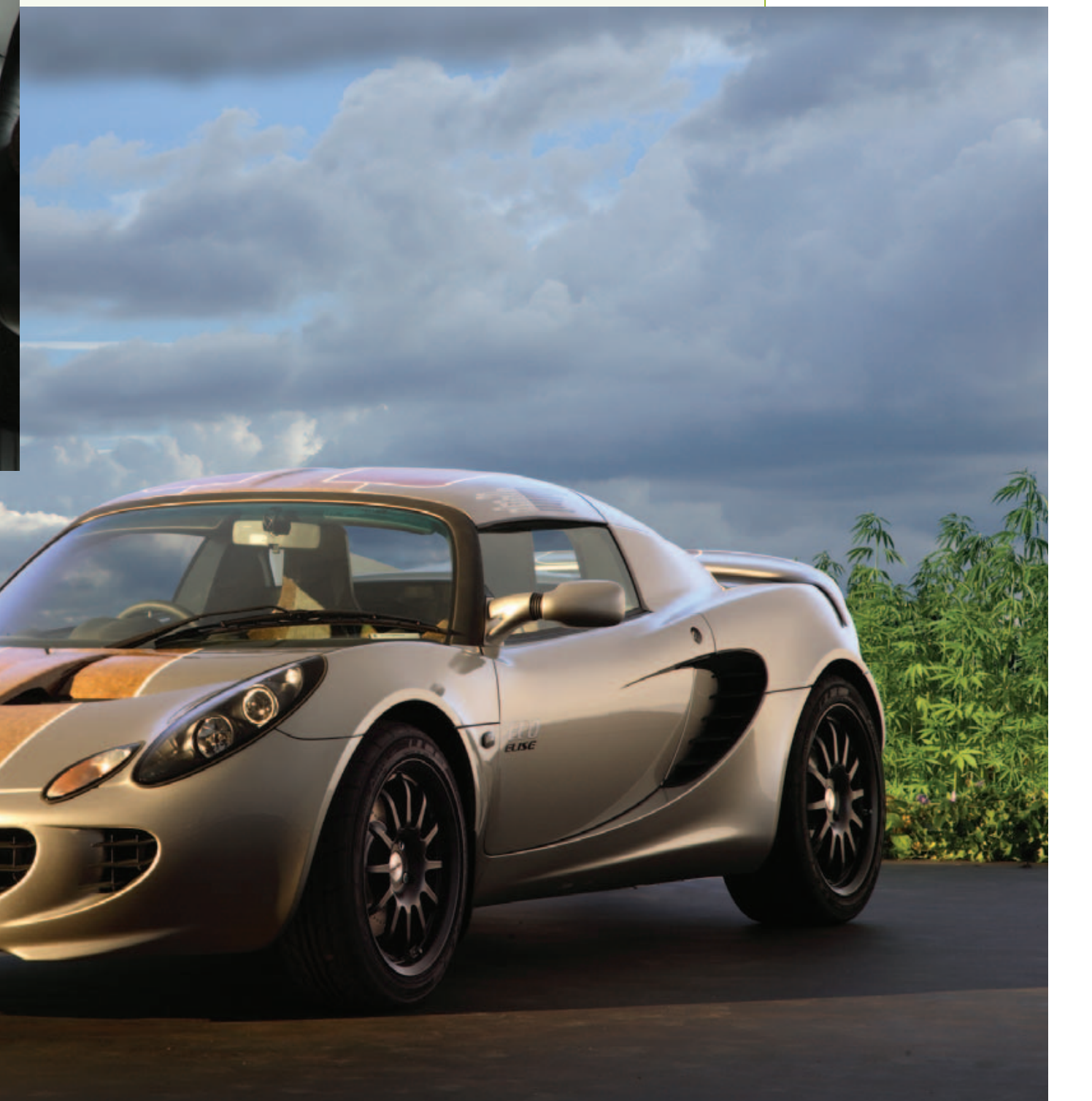
Sports car Lotus Eco Elise, in the main made from different natural fibre compounds, hand lay-up, vacuum bagging and RTM (UK). Pictures: Lotus Cars
