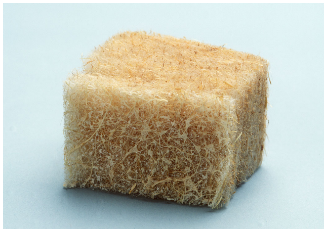
Fig. 20. Spun, loosely compacted hemp insulation. (Manufactured by La Chanvrière de l’Aube, France.)
