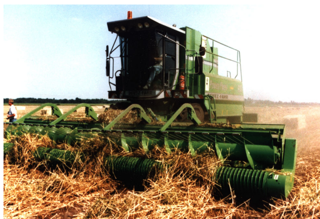
Fig. 45. A hemp harvester operated by HempFlax (Netherlands), with a wide mowing head capable of cutting 3 m long stems into 0.6 m pieces, at a capacity of 3 ha/hour. (Courtesy of HempFlax, Oude Pekela, The Netherlands.)
