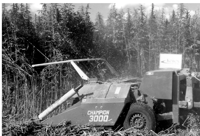
Fig. 44. A John Deere Kemper harvester, with circular drums that cut and chop hemp stalks, shown in operation in southern Ontario. (Courtesy of Kenex Ltd., Pain Court, Ontario.)
