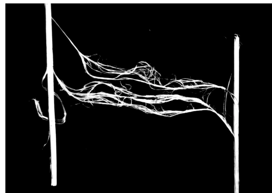
Fig. 14. Fiber in retted hemp stem. This stem was bent sharply after retting, breaking the woody central portion (hurds), leaving the bark fibers unbroken. The two portions of stem are separated in this photograph, and are joined by the tough bark fibers.
