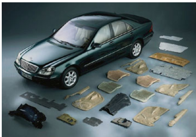
Fig. 18. C-class Mercedes-Benz automobiles have more than 30 parts made of natural fibers, including hemp. (Courtesy of T. Schloesser, Daimler-Chrysler.)
