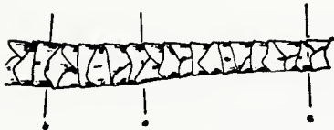
FIG. 4.—Marking Wedge Ruler Where Fiber is not of Uniform Diameter.
